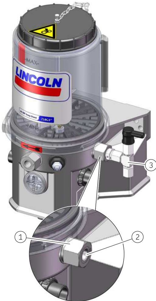
Replacing pump element and pressure limiting valve
