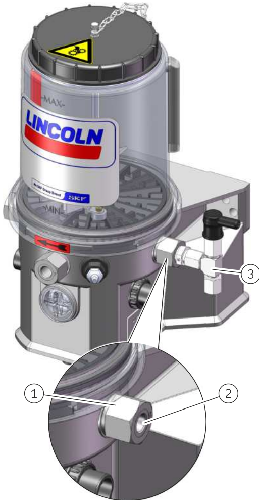
Replacing pump element and pressure limiting valve
