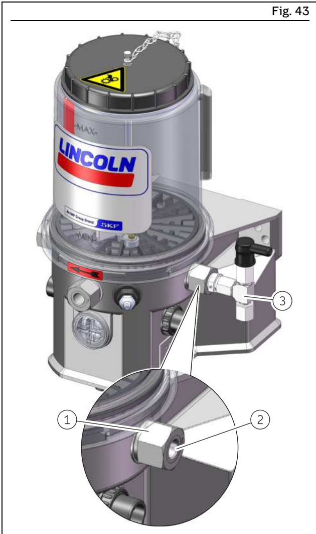
Replacing pump element and pressure limiting valve
